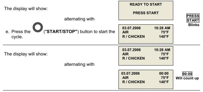
The **AUTOMATIC** mode uses both the food probe and air probe temperatures to control the cycle. When the food temperature has reached the final setting of 40° F, the unit will automatically go into holding mode and a beep will sound for 5 seconds. The elapsed time and food temperature readouts will blink.
