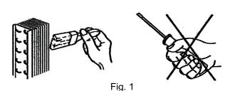
This operation (to be performed every 30 days, max.) can be accomplished using a brush (non-metallic) to remove all the dust and dirt from the condenser fins. Remove the finned grid to gain access to the condenser.
