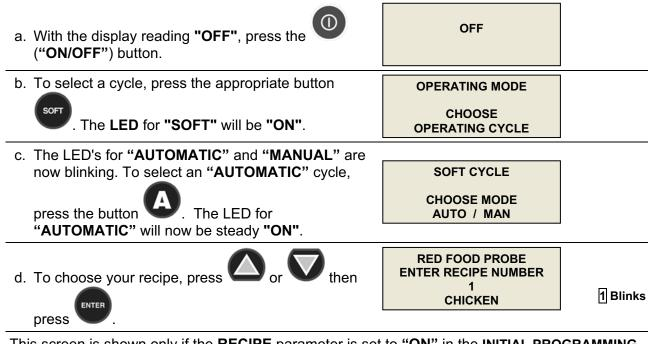
This screen is shown only if the **RECIPE** parameter is set to "**ON**" in the **INITIAL PROGRAMMING**. The red food probe **only** will be active in the standard configuration.
