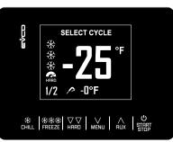
**Soft Chilling:** The air temperature is held in the range of 28°F to 33°F, ideal for delicate food items. The chilling cycle is completed when the food core temperature reaches 38°F.
