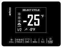
**Soft Chilling:** The air temperature is held in the range of 28°F to 33°F, ideal for delicate food items. The chilling cycle is completed when the food core temperature reaches 38°F.
