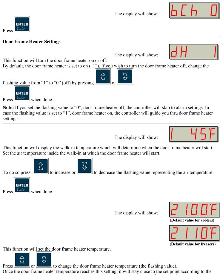
factory set differential. Note: Set the door frame heater temperature between  $75^{0}$ F and  $120^{0}$ F.
